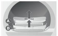
Pull both filters out of the filter holder.
