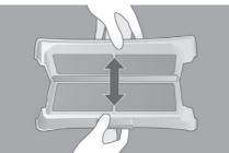
Pull out the outer coarse filter
