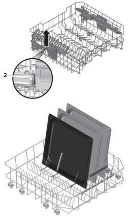
When the upper basket is put back, the basket safety lock 2 must be returned to the locking position.
